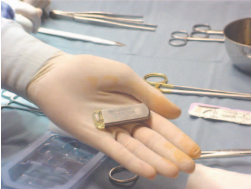
Figure 31.5 Implantable loop recorder. The implantable loop recorder (Reveal) is placed subcutaneously under local anaesthesia, and has a battery life of 18–24 months. The device has a solid-state loop memory, and the current version can store up to 42 min of continuous single-lead electrocardiogram. Retrospective ECG allows activation of the device after consciousness has been restored. Automatic activation is also available in case of occurrence of predefined arrhythmias.
