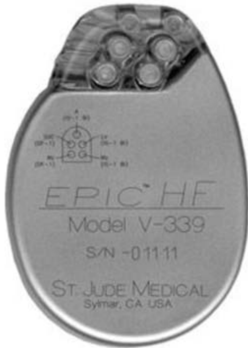
Figure 33.5 Example of a three-chamber implantable cardioverter-defibrillator (ICD) capable of providing cardiac resynchronization therapy in addition to anti-bradycardia and anti-tachycardia stimulation, cardioversion and defibrillation (size, 36 cc; weight, 73 g; maximal high energy output, 30 J).
