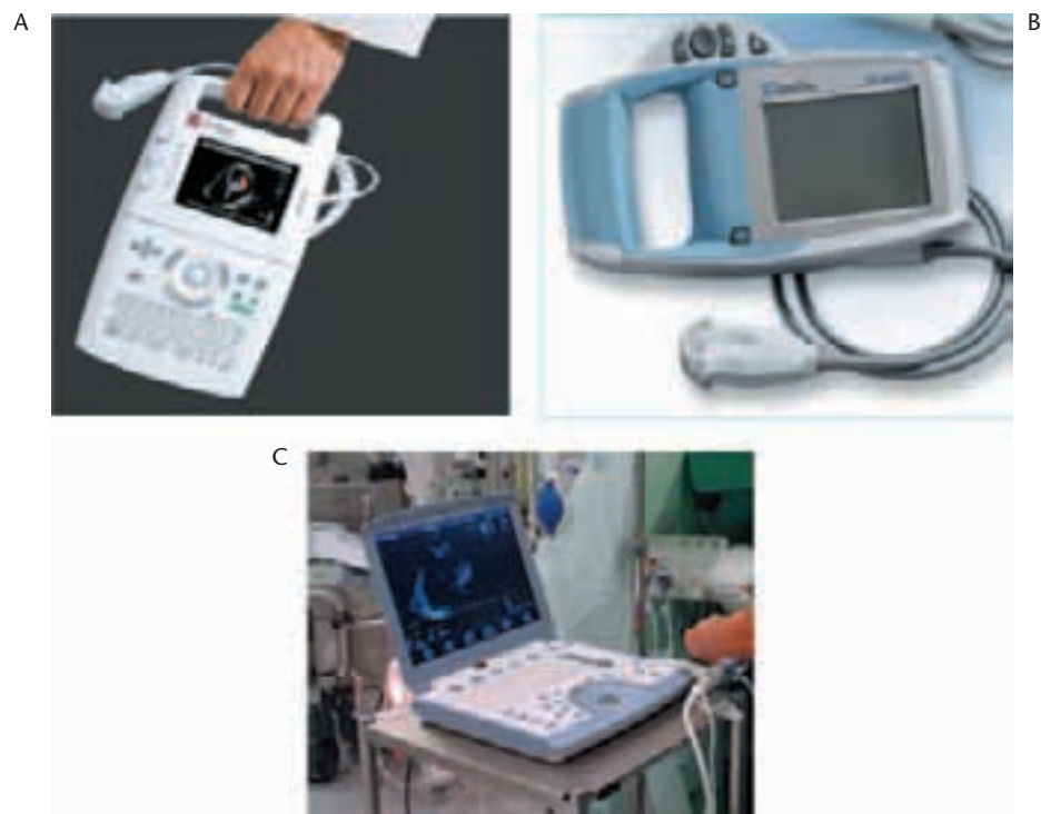
Figure 2.13 Currently available hand-held ultrasonic imaging systems: (A) Sonoheart (Sonosite, Inc.); (B) iLook (Sonosite, Inc.); (C) a recent laptop-based full-featured Vividi (General Electric) system which is available with transthoracic and transoesophageal imaging probes.
